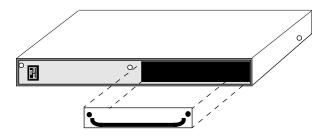
Figure 2-5 Removing the FN10 Backplate
